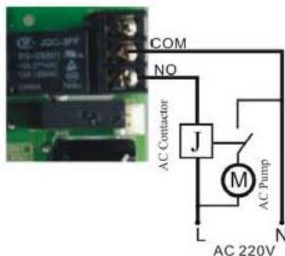
Figure 3-8 Wiring of Booster Pump on Inlet
