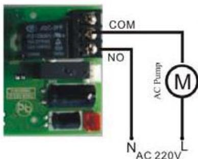
Figure 3-7 Wiring of Booster Pump on Inlet
