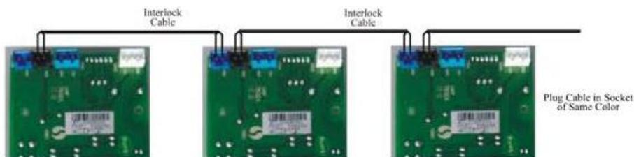
Figure 3-9 Network System Wiring with Interlock Cable
