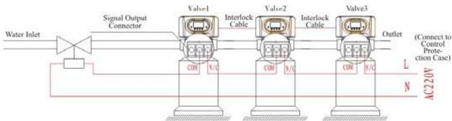
Figure 3-4 Wiring of Solenoid Valve in Inlet
