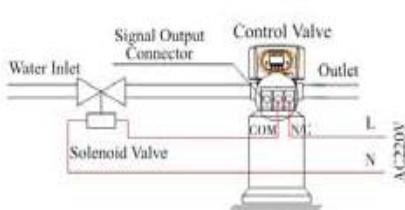
Figure 3-2 Wiring of Solenoid Valve on Inlet
